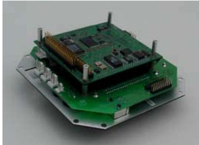
*Elektra CPU board mounted on panel board*
