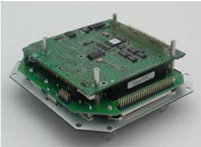
*Athena CPU board mounted on panel board*
